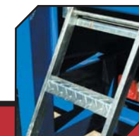
FOLDAWAY STEP LADDER Enables easy access to the trailer for the operator
