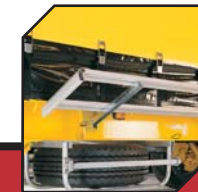
SPARE WHEEL CARRIER SDC standard fully galvanised security double or single wheel carrier can be bolted into position forward or behind axle bogie
