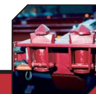
14 LOCKS STANDARD ON EXTENDABLE For carriage of all combinations of container & intermodal bodies
